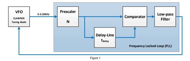
The circuit has a negative feedback loop that acts on the VFO. For frequency correction, the capacitance diode built into the VFO (primary for CLARIFIER) is also used.
