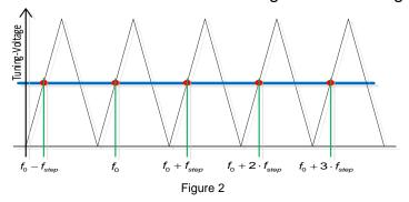
If e.g. and  $t_{delay} = 0.2s$  amount N = 2, then the FLL step size will  $f_{step} = 10Hz$  be. Mathematically derived, the lockup point can be calculated as follows:
