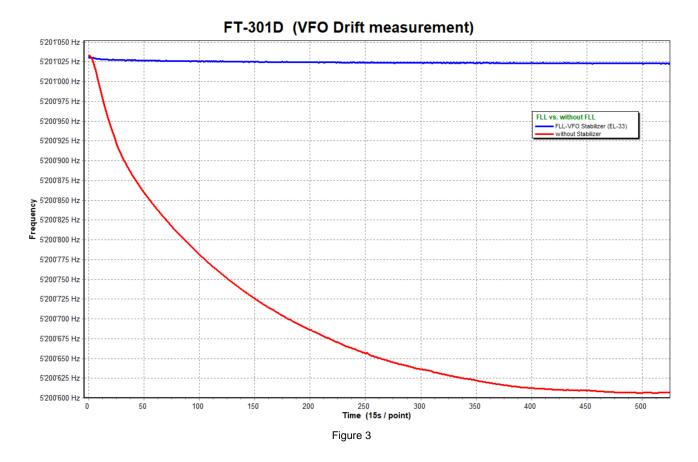
The effect of the FLL-VFO stabilizer can be seen in Figure 3. Measurements were taken over a period of approx. 2h (525 x 15s) after switching on the FT-301D. Without stabilization the VFO drifts about 425Hz. Such a strong drift is extreme annoying in CW or SSB mode, and digital modes are unthinkable.
