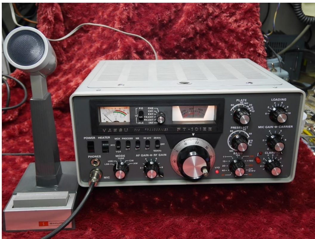
Figure 1- FT-101 after EL-34 modification
