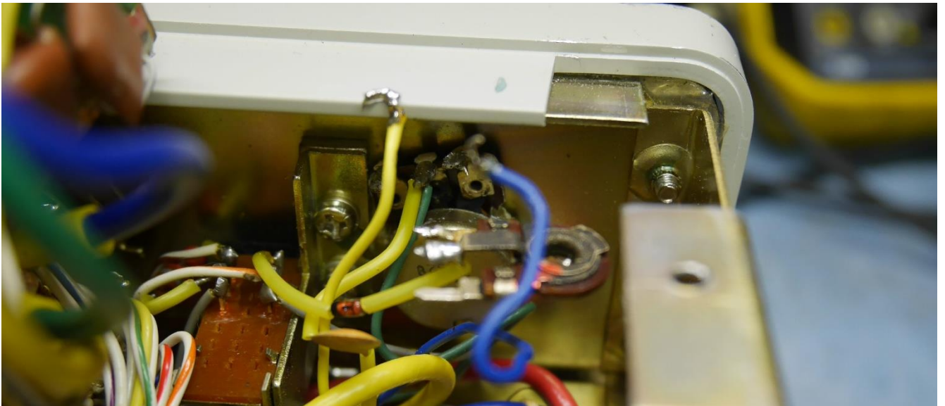
Figure 9- desoldered zero-point potentiometer and the two wires
