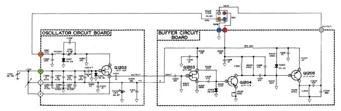
Figure 2- Heathkit VFO Schematic
