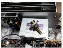
Figure 3 - Outer Shaft Coupler
