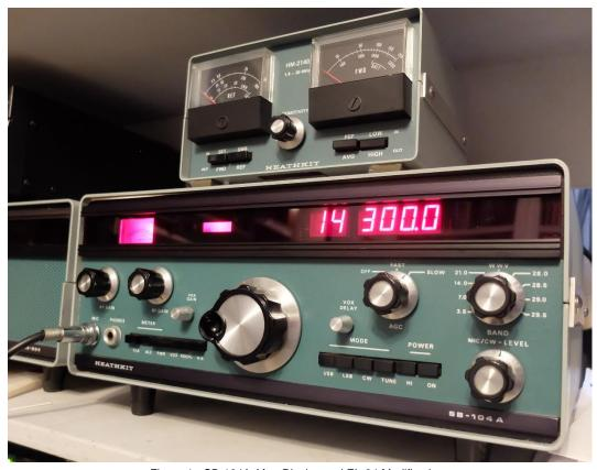
Figure 1 - SB-104A After Display and EL-34 Modifications
