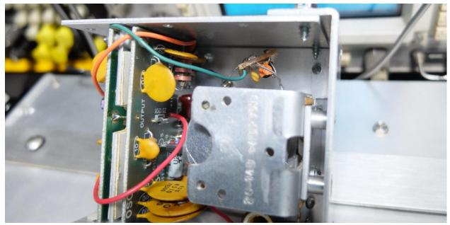
Figure 7- Installed Varactor Circuit Board
