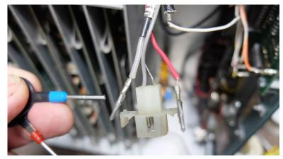
Figure 8 - Pin Removal
